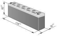
N.B. Always observe the polarity during installation (red = positive, black = negative). If the battery is flat and its voltage is lower than 10.5 V, the siren stops sounding, while the light indicators remains on.
