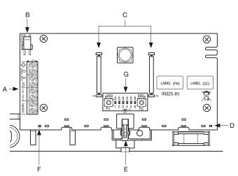
A: Connection terminals (see the TERMINALS figure for details)
