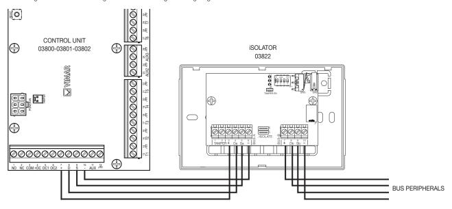
Simply use the isolator art. 03822 with the two connected jumpers (default). In this case, the BUS towards the field peripherals is regenerated and the power supply conductors + and - are the same as the control unit. The BUS signals are on the other hand regenerated, isolated and protected. Install the isolator in an enclosure which is in turn protected.
