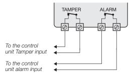
To detect sabotage/tampering, you need to connect the related signal to the terminal configured as MAINTENANCE type GENERAL ZONE
