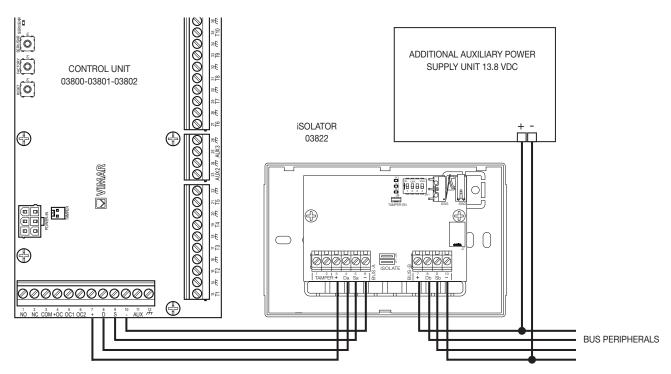
In this case, the isolator art. 03822 is still used but the two jumpers need to be cut. The power supply of the BUS peripherals is galvanically isolated from the control unit and is supplied by the auxiliary power supply unit. The maximum current available depends solely on the characteristics of the auxiliary power supply unit itself.
