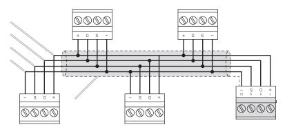
The sizing of the BUS line, in other words the distribution of the peripherals and the use of cables to connect them, should be done according to various design factors, in order to guarantee the correct transmission of signals of the "D" and "S" conductors and of the power supply provided by the "+" and "-" conductors.
