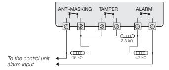
The table below shows the values (expressed in  $\Omega$ ) of the equivalent resistor read at the terminals according to the balancing and signal detected. The table applies to EOL resistors supplied by default, which are  $3300\Omega$ ,  $4700\Omega$  and  $15000\Omega$ .
