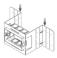
The bracket must be fixed using the holes closest to the bracket base bend (if necessary using suitable adaptors such as screwdriver extensions, etc.).
