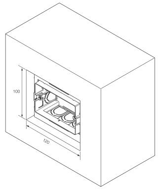
Use fixing foams, fill the empty space behind the mounting box. Lastly, trim the front.
