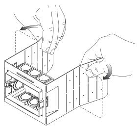
Bend according to the dimensions indicated on the product label depending on the height at which you wish to position the mounting box.
