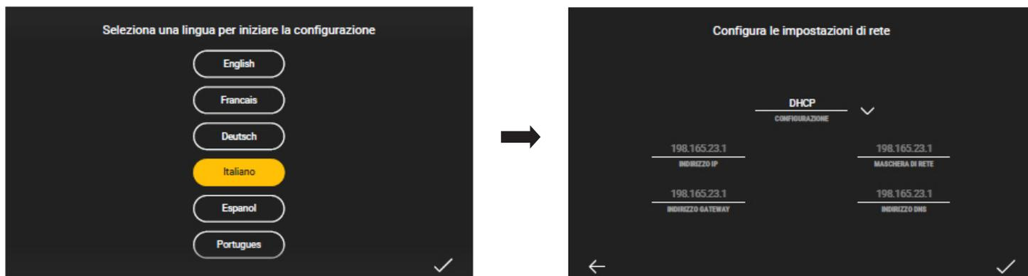
By default the system is set to DHCP and so configuration is automatic (recommended choice); vice-versa, if you need to enter the network parameters manually touch
