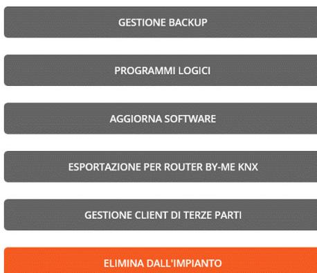
**IMPORTANT:** the "EXPORTING FOR BY-ME KNX ROUTER" option can only be used for home automation system gateways 01410-01411.
