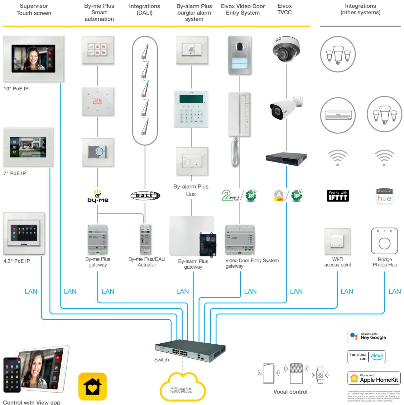
We recommend you use high-performance switches that guarantee the reliability of the IP-based platform (for instance Elvox switches). Avoid using the ports of consumer routers, because the type of filtering that may be applied to transiting data is not known in advance.
