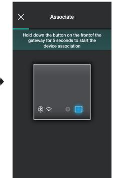
• Press the front push button on the gateway for 5 s.
