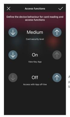
Access with App off-line: allows you to use the View Key App to open the gate in places where the smartphone does not have Internet connectivity (for instance in a cellar or basement).
