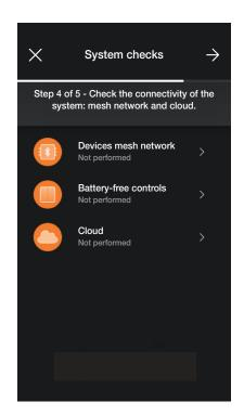
• Select "Devices mesh network" to activate the test to make sure the wireless connection between the gateway and all the devices (electronic 2-way switch, control device with relay output and roller shutter control device) are working properly.
