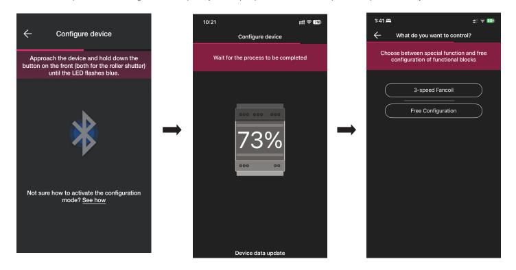
Use the "3-speed fan coil" and "Free configuration" options to define the behaviour of the various outputs.
