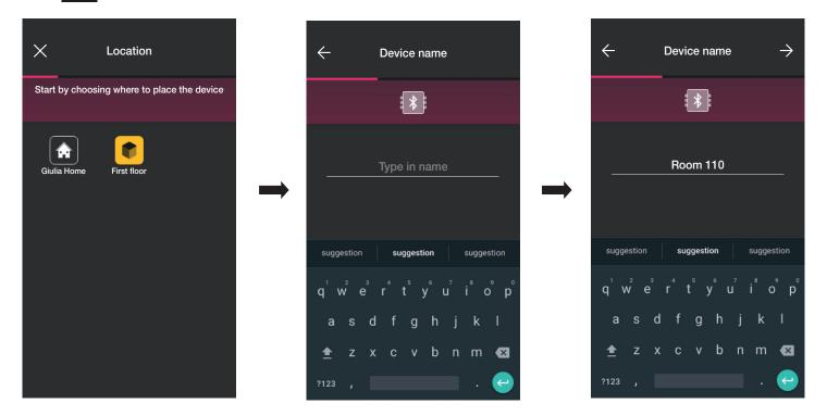
• Select to confirm; with the Bluetooth connection active, approach the reader and press the configuration push button. Once the device has been detected, the Approach recognises whether it is a landing reader or a pocket (in this case it is a landing reader).
