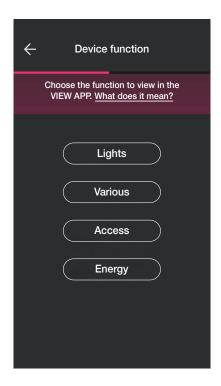
• Select "Energy", the App will prompt you to update the firmware to the latest version (only where necessary) and to set the colour of the LEDs and the brightness level.
