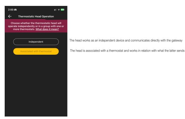
N.B. The head is inserted in the Bluetooth mesh network and therefore needs at least one mains powered IoT device (control, etc.) to be within its radio range. The head cannot operate in stand-alone mode.
