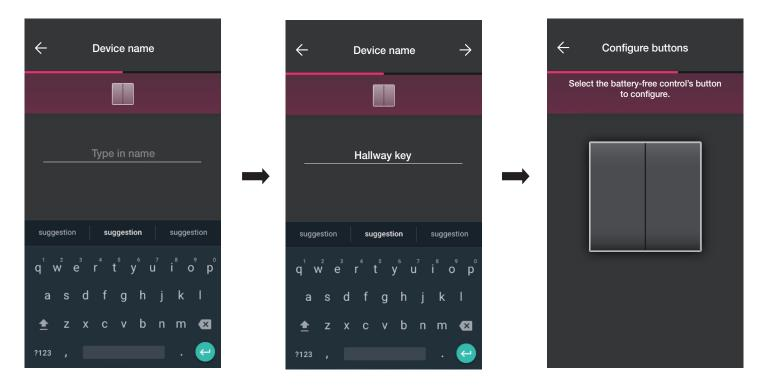
• Press the button you wish to configure on the radio control 03925; the App will display the chosen button. The next screen displayed is to choose whether to use the button to replicate the function of the device (in this case the 2-way switch) with which the radio control has been associated to call up a generic scenario.
