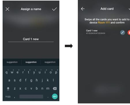
The operation illustrated above should be repeated for all the cards to be associated with the entrance; once the association process is complete, confirm with
