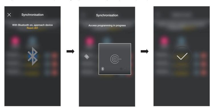
This procedure should be repeated for all the devices containing cards to be replicated; at the end, the Access management screen will be displayed.
