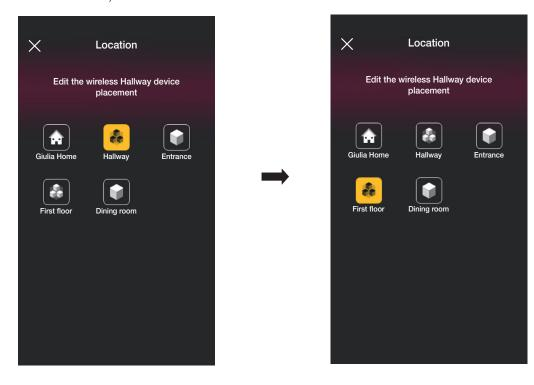
If the device is associated with a sub-environment, the main environment will be displayed in yellow; the device may therefore be moved there or to another environment or sub-environment in the system.
