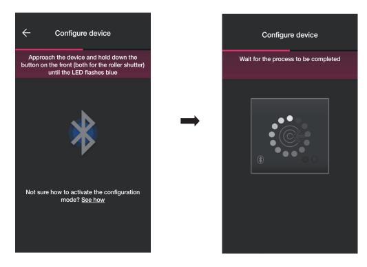
• When the process is complete, the App checks the firmware version on the device and, if it is not the most recent, the update is performed.
