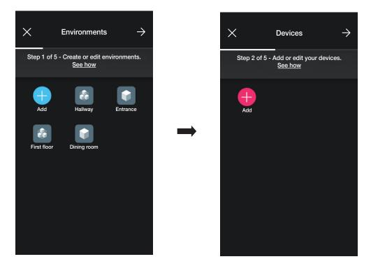
• Select (Add); choose the environment in which to place the device (for instance "FIRST FLOOR") and assign a name to it.
