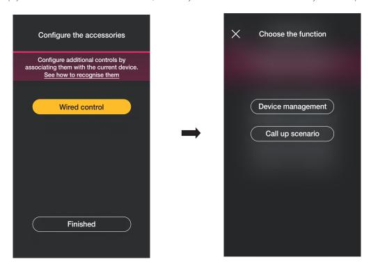
Select "Device control" for the wired push button to control the relay.
