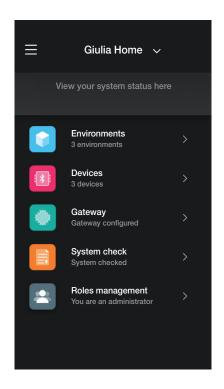
The management screen allows you to View the system by environments and sub-environments or by devices with all the associated functions.
