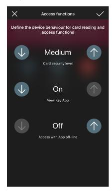
Access with App off-line: allows you to use the View Key App to open the gate in places where the smartphone does not have Internet connectivity (for instance in a cellar or basement).
