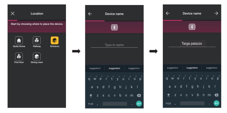
• Select  $\rightarrow$  to confirm; with the Bluetooth connection active, approach the entrance panel and activate its configuration mode.
