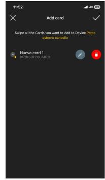
The operation illustrated above should be repeated for all the cards to be associated with the entrance; once the association process is complete, confirm with
