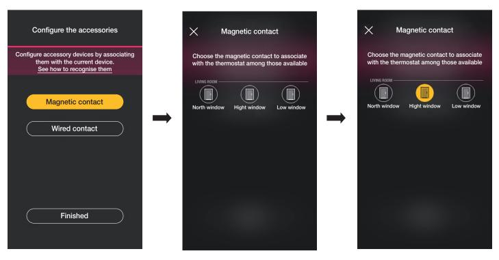
The App will complete the association and the thermostat will be associated with the "High window" contact (in the case an open window, the notification will be sent and the temperature control will be interrupted).
