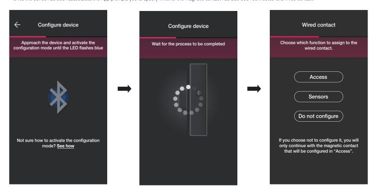
By selecting "Acess" the wired contact can be used to detect the opening of a door or window.
