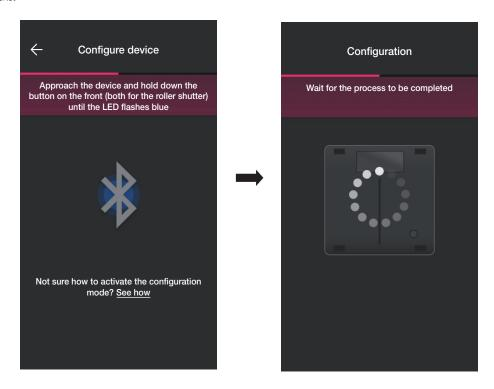
• When the process is complete, the App checks the firmware version on the device and, if it is not the most recent, the update is performed.
