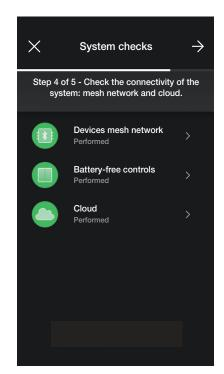
If the test has "Failed" the respective icon will be in red (for instance ); the icon will instead be orange (for instance ) if the test could not be performed.
