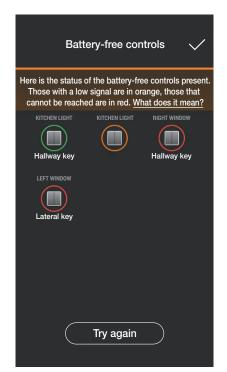
At the end of the test, all the controls art. 03925 and the respective environments will be displayed; those with a good signal will be displayed in green, those with poor quality signal in orange and those not reached or with insufficient signal in red. Select "Try again" to repeat the test.
