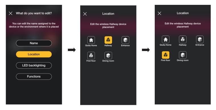
If the device is associated with a sub-environment, the main environment will be displayed in yellow; the device may therefore be moved there or to another environment or sub-environment in the system.
