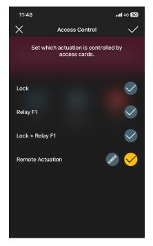
• Select of "Remote actuation" (after enabling it) to set the parameters which define its function.
