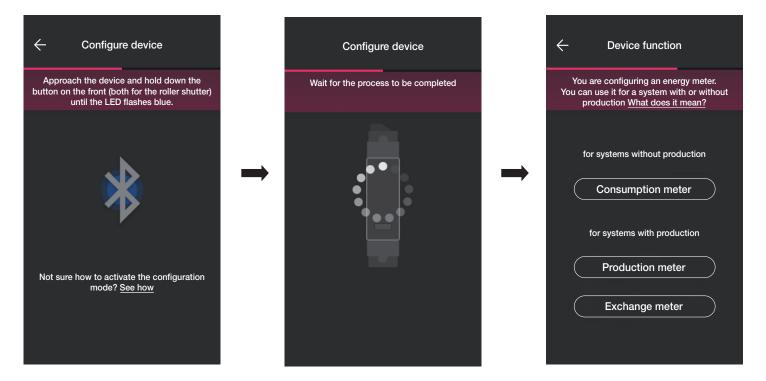
• Once you have associated the device, depending on the type of system (without production or with production), select the type of metering to perform and confirm with
