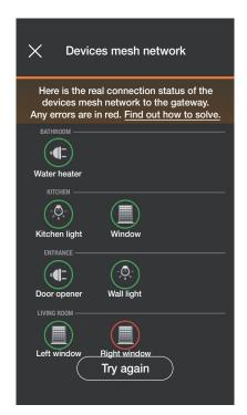
At the end of the test all the devices (wireless nodes) and respective environments will be displayed; those reached correctly will be displayed in green whereas those with which the gateway was unable to establish a connection will be displayed in red. Select "Try again" to repeat the test.
