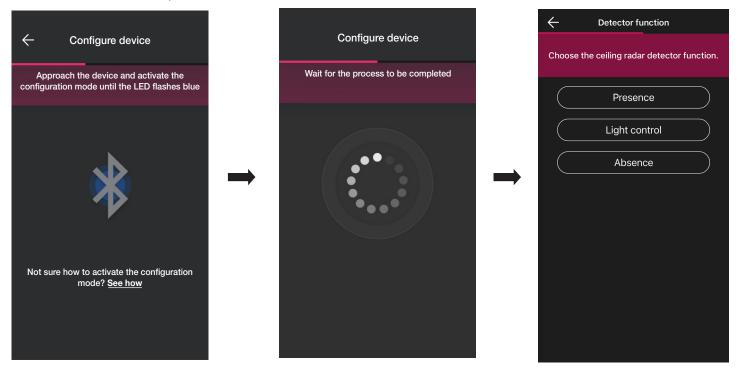
• Set the actuators connected to the status of the relay on board the sensor (those available according to the chosen function will be displayed).
