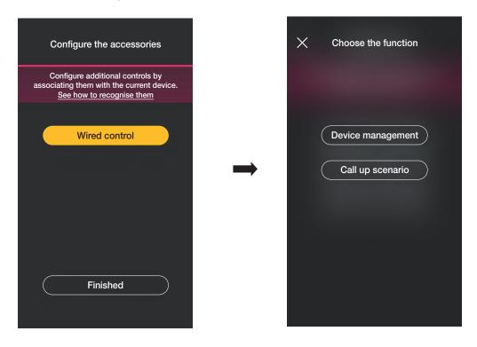
Select "Device control" to replicate the function achieved by the sensor (relay control) without further options.
