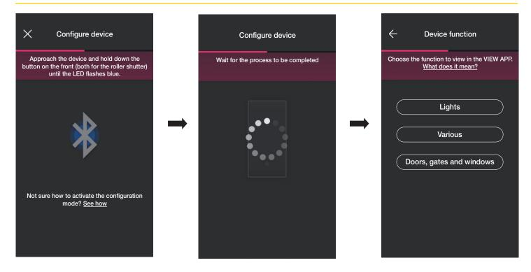
• Once you have associated the 2-way switch, select the function (in this case Lights) and confirm with \_\_\_\_. The LED backlighting and the parameters will be set subsequently as illustrated in para. 2.2.
