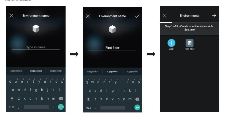
Every environment created can in turn be divided up into other sub-environments (up to three depth levels); this option is useful in the case of systems with many devices or to divide up the system down to the smallest detail. The creation of sub-environments is optional and can therefore even be omitted.
