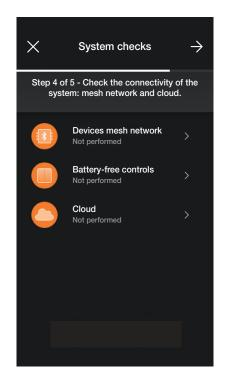
• Select "Devices mesh network" to activate the test to make sure the wireless connection between the gateway and all the devices (electronic 2-way switch, control device with relay output and roller shutter control device) are working properly.
