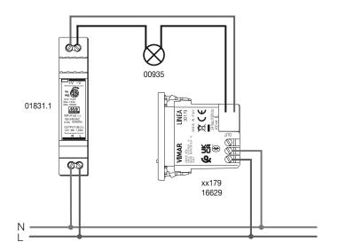
3. Connection to control switchboard or to device with potential-free inputs
