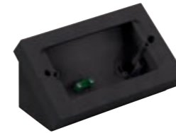
▲30784.G Tilted table mounting box, with variable height, for the installation of 4 modules. In the lowered version, connector blocks with a maximum depth of 32 mm can be installed; if you turn the cover the maximum depth extends to 44 mm. The socket outlet with USB, 30210, USB, cannot be installed. To be completed with mounting frame and cover plate.
