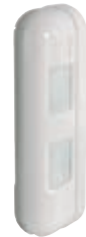
01739 Passive infrared presence detector for the protection of building exteriors, 12-metre curtain-effect detection on each side (left and right), PET immune, IP55, 1 input for acoustic control, 2 NO and NC 28 Vdc 0.2 A relay outputs, surface mounting, 10-28 Vdc 38 mA power supply
