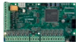
▲03800 By-alarm Plus control unit expandable to 25 zones
