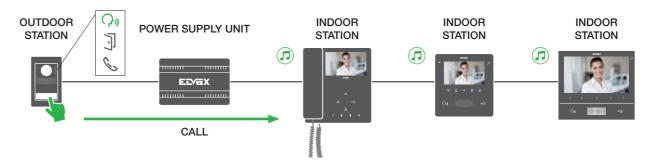
The first indoor station that answers by lifting the handset or pressing the talk/listen button will begin communicating with the outdoor station, while the others will stop ringing and generate the engaged tone.
