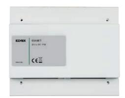
The video selector for 4 cameras 69AM/T allows the connection to the Due Fili Plus system of 4 cameras with CVBS output. Camera selection is cyclical by way of the lock release button or a dedicated push button after the self-start phase. The selector can also be connected to two auxiliary functions F1 and F2.
