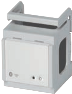
OK14597.01 Wi-Fi Bluetooth® wireless technology gateway for integration, configuration and supervision of View Wireless system by Cloud and app for smartphone and tablet, 100-240 V 50/60 Hz power supply, on DIN (60715 TH35) rail installation, occupies 2 17,5 mm modules
