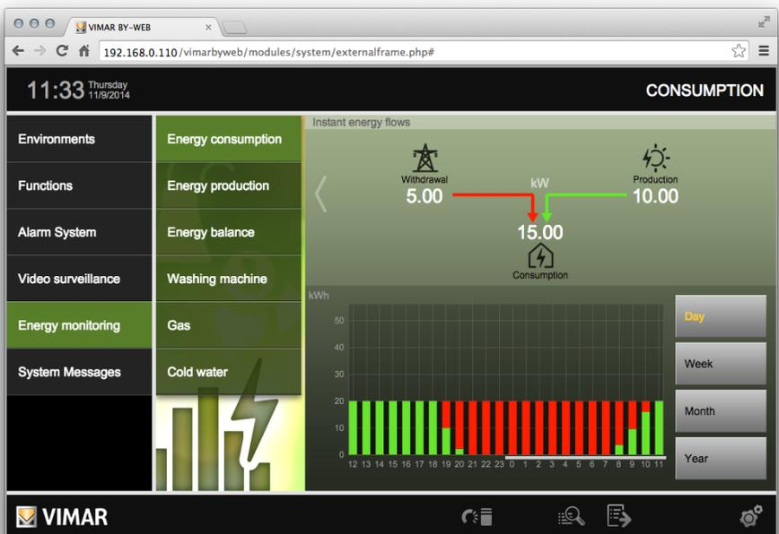
The instant energy flows pattern, shows, in real-time, instant values, in KW, of the consumption of electricity drawn off from the public network, the production of photovoltaic energy, the amount of energy input into the public network and the total consumption of the loads.
