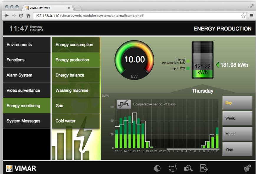
At the top right corner of the page, the stack diagram represents the overall production since the beginning of the reference period (current day / week / month / year); the reference period is highlighted below the graph bar by a white line. The total value is shown above the diagram.
