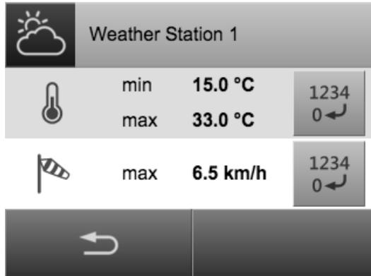
The first row shows the minimum and maximum temperature, followed by the button to reset these values. The second row shows the maximum wind speed, followed by the button to reset these values.
