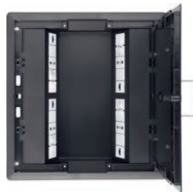
↑ ↑ 4 side connector block compartments for 5 modules each. The two adjacent compartments are separated by a dividing screen to be used for different systems. If you want to dedicate the 10-module row to the electrical components, simplifying installation and wiring, you can remove the dividing screen
